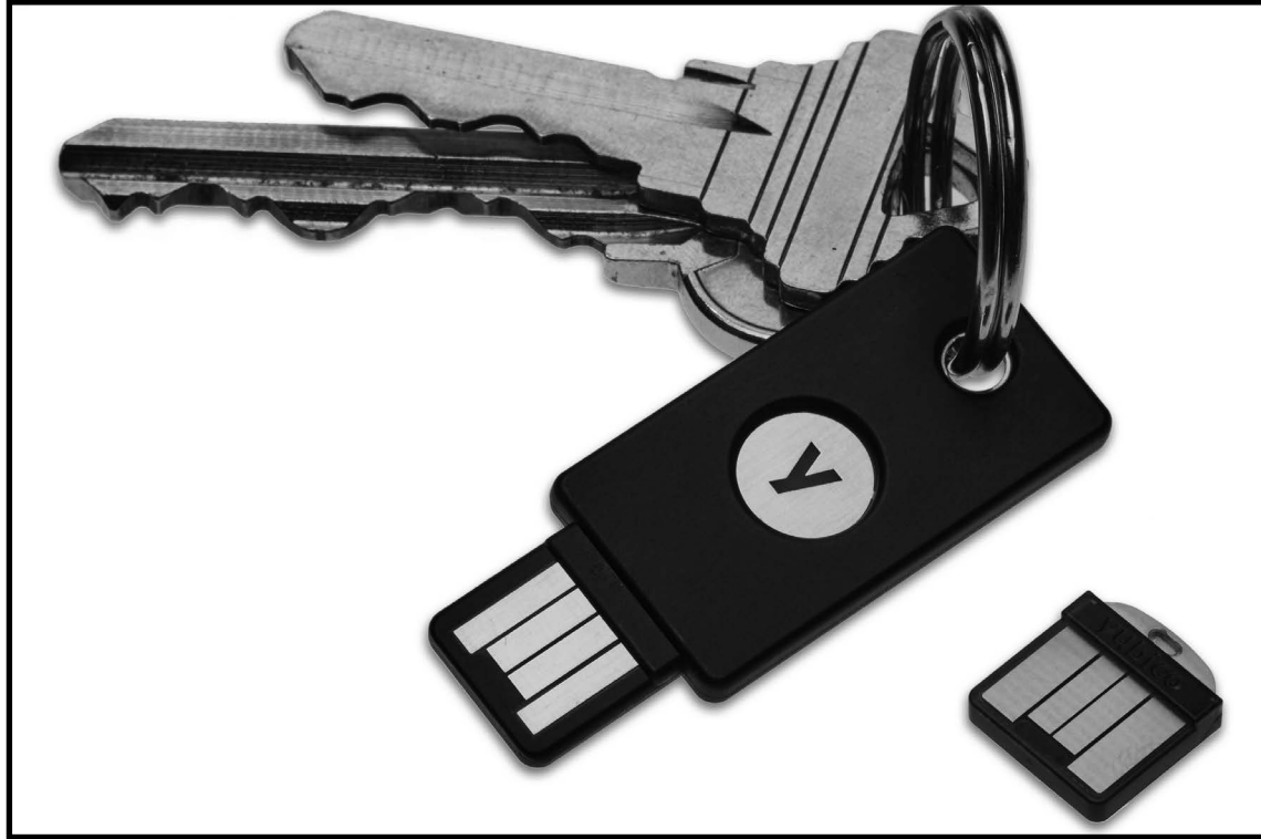
A Yubikey, which provides an alternative token to phones for two-factor authentication. Photo courtesy Wikipedia.
